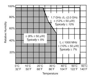
Measurement Range RF IN/OUT<sup>1</sup> 100 MHz <f<sub>C</sub> <2.0 GHz:
